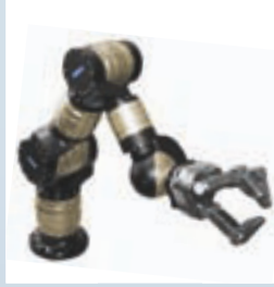
7 DOF LWA4-Arm with 10 kg payload*
