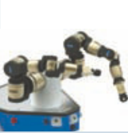
6 DOF LWA-Arm with 4 kg payload*
