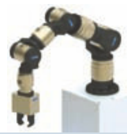
7 DOF LWA-Arm with 3 kg payload*
