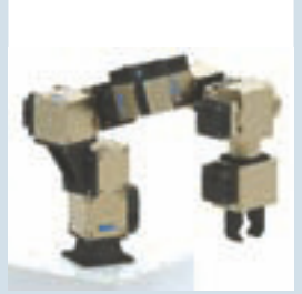
6 DOF PBA-Arm with 3 kg payload*
