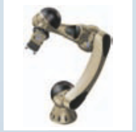
6 DOF PBA-Arm with 3 kg payload*
