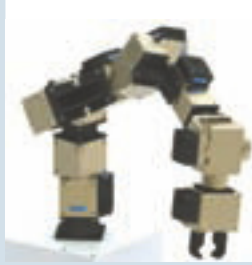
7 DOF LWA4-Arm with 10 kg payload*
