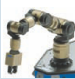
7 DOF LWA-Arm with 10 kg payload*
