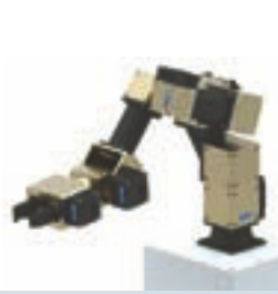
7 DOF LWA-Arm with 3 kg payload*
