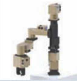
6 DOF LWA-Arm with 4 kg payload*
